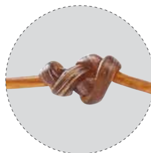
Twisted multifilament with a monofilament appearance
