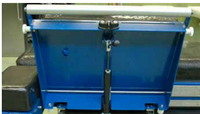
Stepless control of side panels by gas hydraulic cylinders
