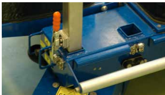
Vertical bars for leg support are locked to frame - cannot be accidentally pushed out
