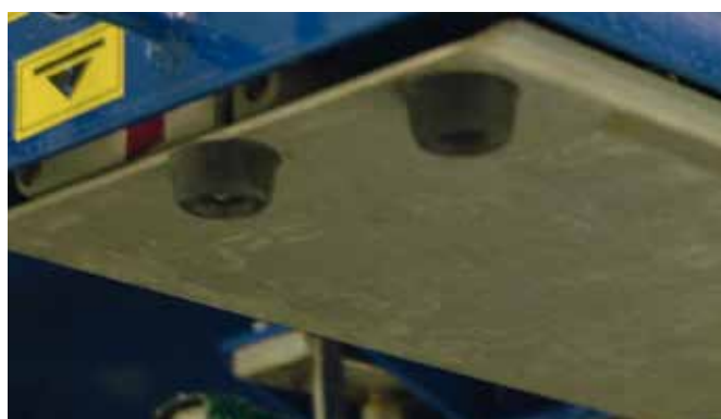
Safety switch under each corner & head support - no leg injury when lowering the table
