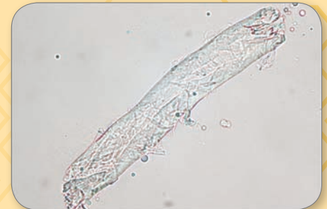
Figure 24 Contaminant fragmented fiber
